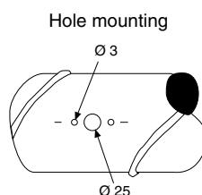
The bracket is used as a template marking up the hole position.
